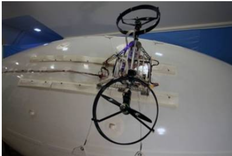
Figure 5: Adjustable Propellers mounted to the Envelope of a Blimp
