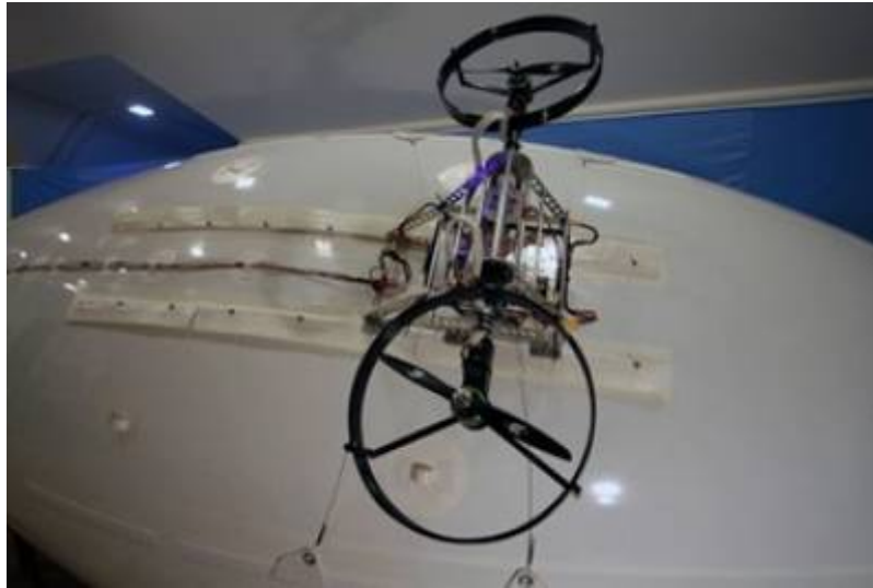
Figure 11: Adjustable Propellers mounted to the Envelope of a Blimp
