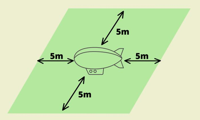
1.The first step to launching our airship is to find a place where it will not meet any obstacles on its way.
